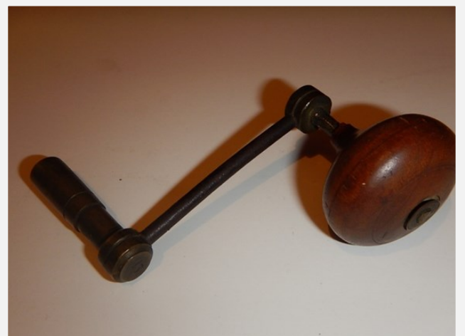
Figure 6. The original hand-forge winding key with the number “13” stamped on the key shaft end.
