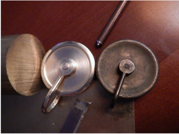
Figure 5. The original pulley (left) and parts used to fabricate a new pulley (center).
