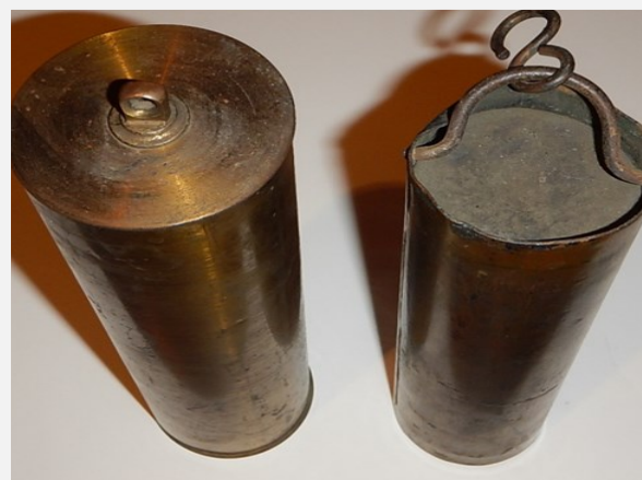
Figure 3. The weights for driving the clockwork and bell mechanisms.
