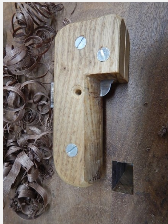
Figure 7. The profiling plane (top) made by Robert McKeown Jr. for finishing the base molding replacement piece (bottom).
