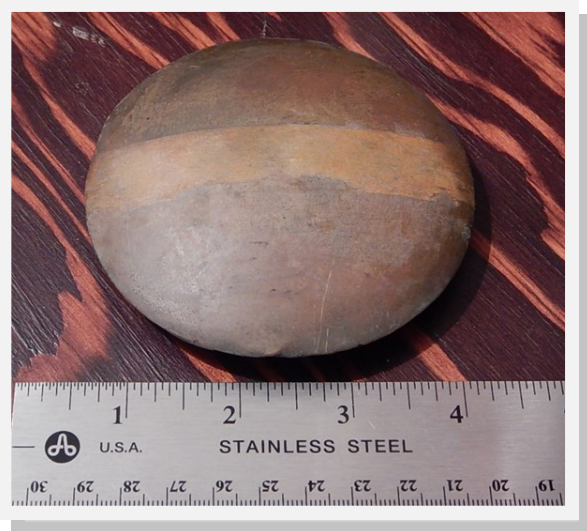
Figure 2. The face of the brass pendulum weight – the stripe is residue from tape which had been used many years ago for storing the weight.
